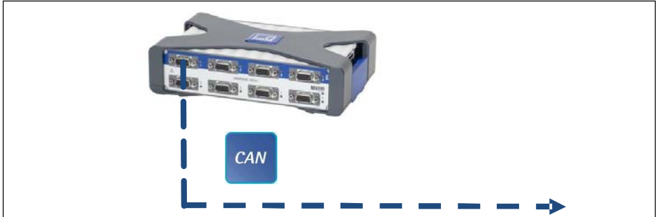
Fig. 7.9 Output to CAN bus (MX840A, connection 1)
